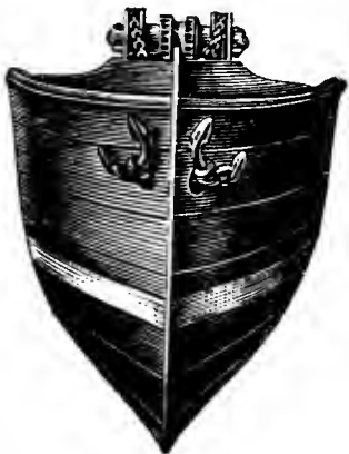
ANCHORS STOWED IN HAWSE PIPES.
